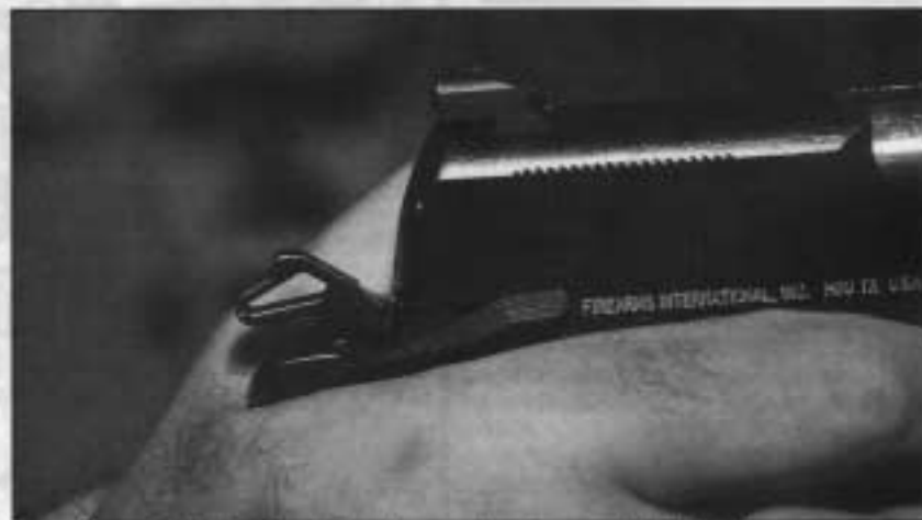
Pressing on the thumb safety releases the hammer to full cock.
