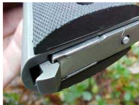
The magazine catch is on the heel, which is a good design for a trail gun.
