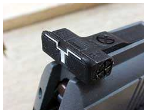
The Automag II is equipped with fully-adjustable, high-visibility Millett style sights.
