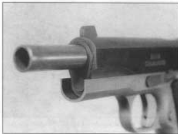
Just as Browning invented it, bushing and standard recoil plug.
