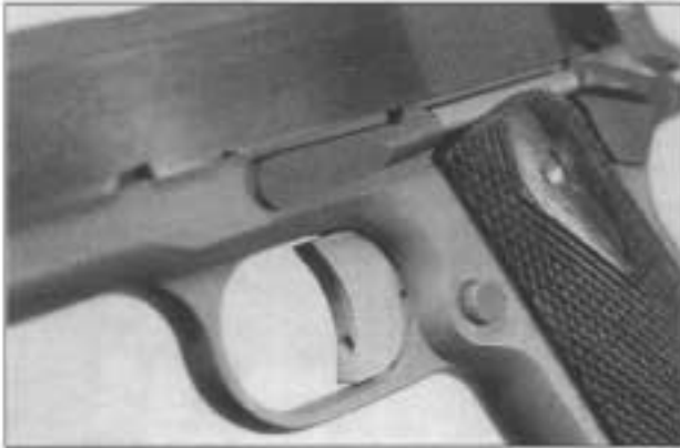
The trigger has an over-travel screw. The slide stop is checkered, the mag button serrated.
