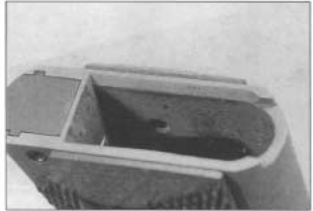
The mag well is beveled, despite the High Standard's plain appearance.
