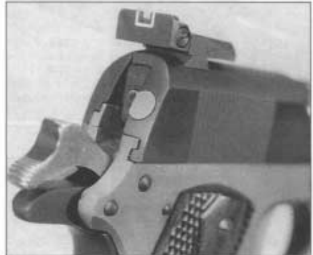
The stainless extractor in the blued slide. For those who like white-outline sights, the High Standard has them.
