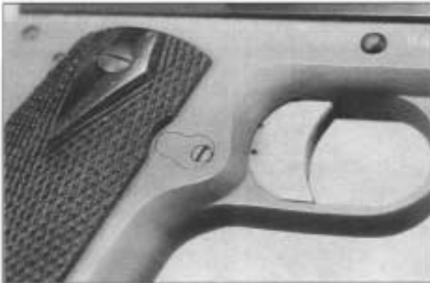
The frontstrap curve is standard, the mag catch button has a slotted head.
