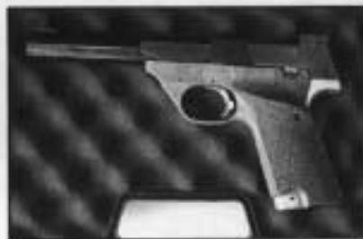
ABOVE: The gold plated High Standard trigger has been a trade-mark on both previous and current models. The set screw through the trigger controls backlash.
