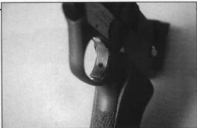
ABOVE: The gold plated High Standard trigger has been a trade-mark on both previous and current models. The set screw through the trigger controls backlash.
